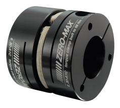
Align the shafts within the limits for parallel and angular misalignment specified on the Table on page 2. For best alignment results, use a laser alignment tool or dial indicator. If not available, a straight edge and feeler gauges can be used.
